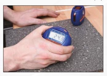
For measuring surface micro-roughness stated as an average roughness figure in microns, RzDIN, which may be useful to assess slip risk
