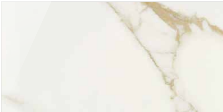
Bianco Oro Polished* CS2242-12060 • 1200 x 600 x 10mm • 23kg per m 2 • Detail variation: 27 Faces CS2242-9090 • 900 x 900 x 10.8mm • 23kg per m 2 • Detail variation: 28 Faces CS2242-6060 • 600 x 600 x 9.5mm • 21.7kg per m 2 • Detail variation: 28 Faces • NEW PEI Rating: 3
